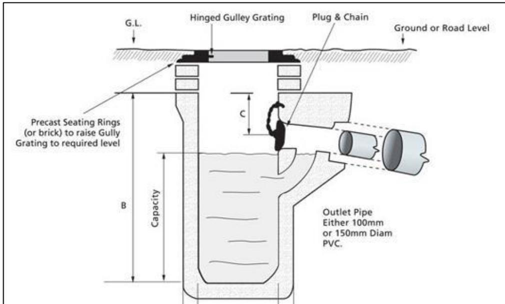
Plate 3-5 Trapped Road Gully (Typical Detail)
