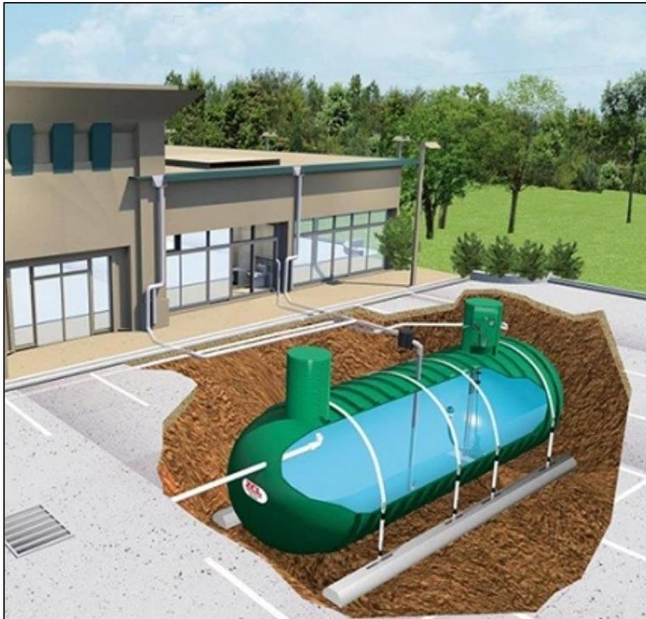
Plate 3-1 Example of Rainwater Harvesting System
