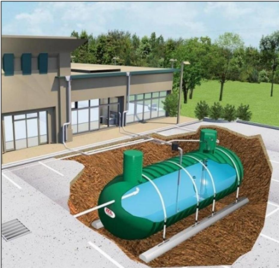
Plate 2-1. Example of Rainwater Harvesting System
