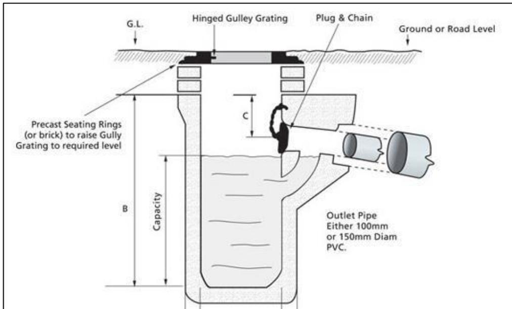
Plate 2-5: Trapped Road Gully (Typical Detail)
